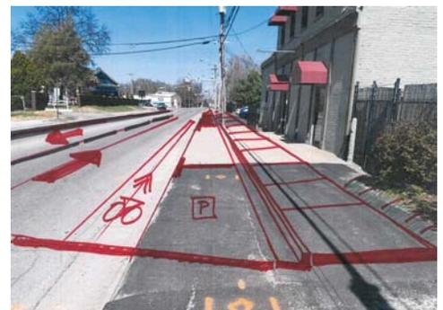
Figure 9: Sketch of proposed sidewalk improvements on the east side of Spring Street north of Riddle St. By reclaiming the paved ROW on the building side of the concrete gutter we can reintroduce parallel parking in this segment.
