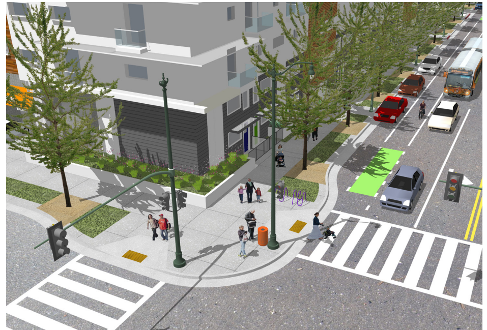
Permanent curb extensions make directional ramps possible on a corner that otherwise would be too narrow. They reduce the crossing distance and increase pedestrian visibility.
